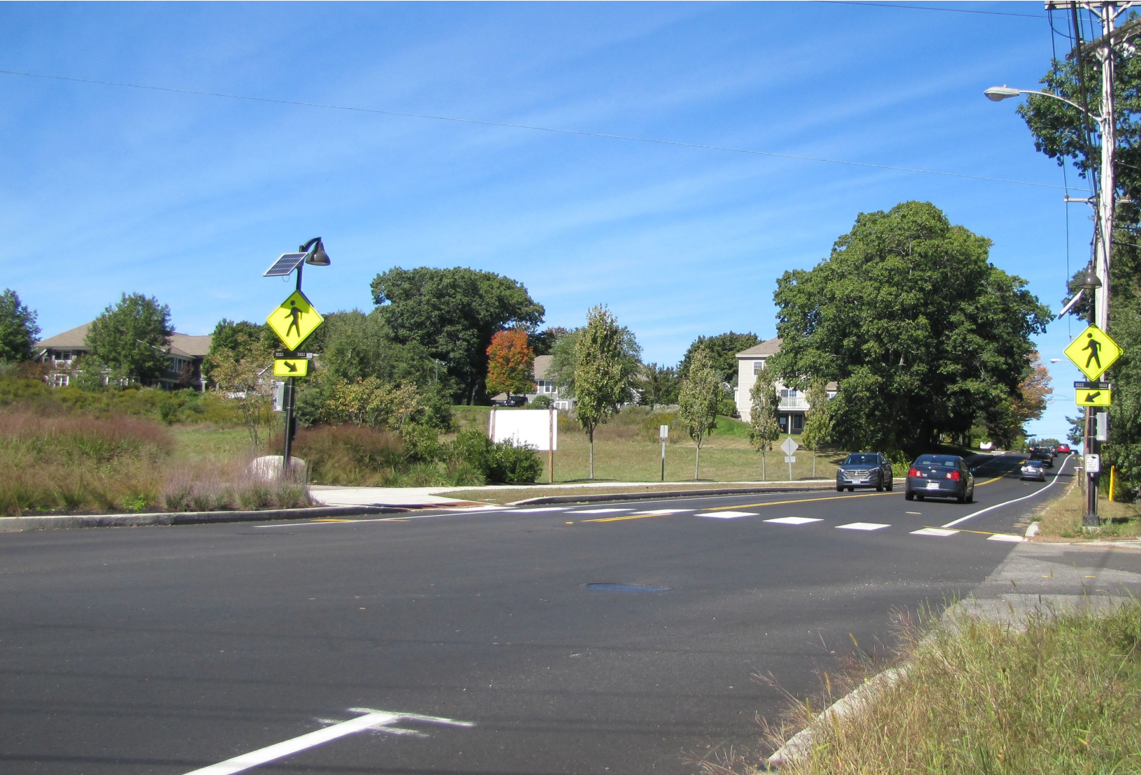
RRFB on Black Point Road in Scarborough. Similar to PHBs, these are pedestrian-activated and support safe crossings. Source: Town of Scarborough
