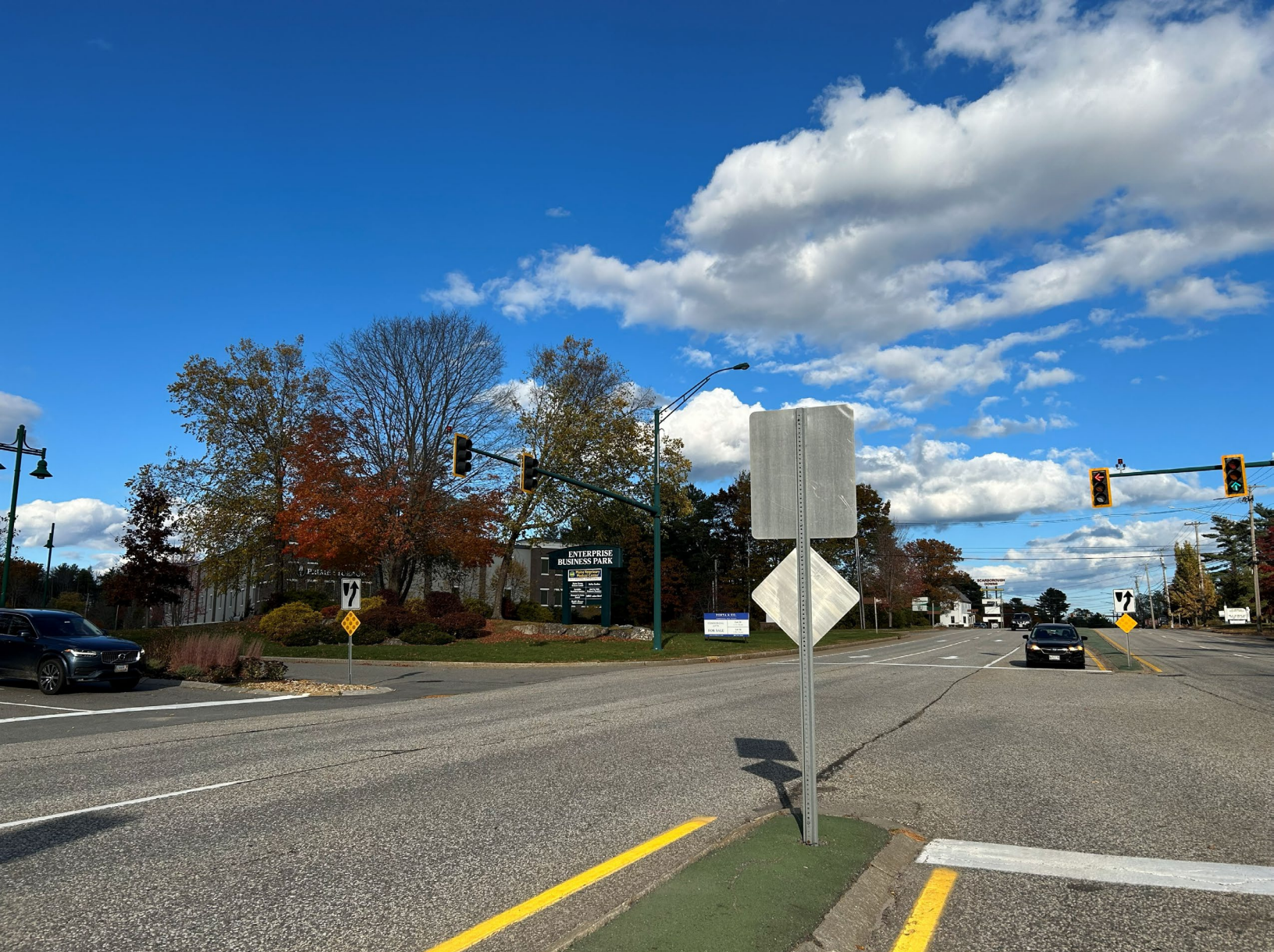
Route 1 in Scarborough is an example of a Major Corridor. Although this street type has high traffic volumes and speeds, tools like the medians shown here can help calm traffic. Source: Nelson\Nygaard
