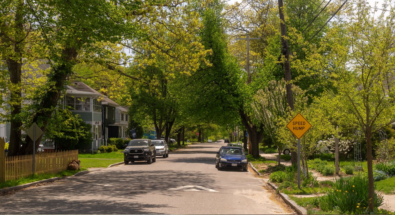
Speed hump in Portland, ME. This tool is ideal on roadways with less public transit and lower traffic volumes. Source: GPCOG
