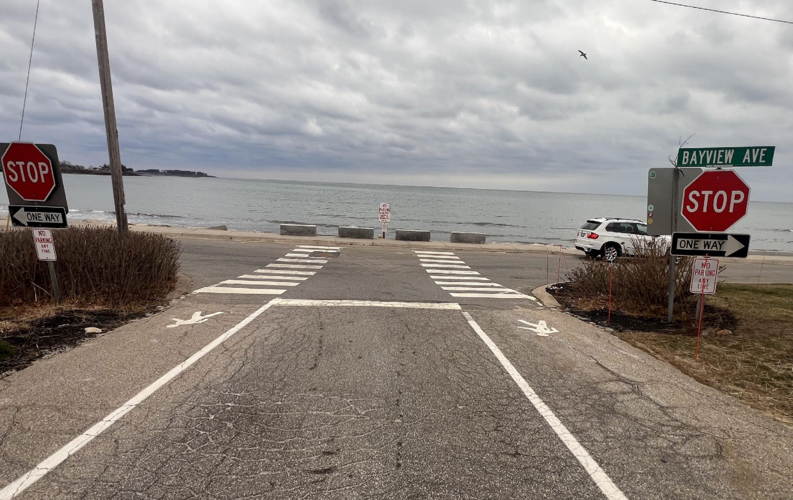
Walking and rolling lanes, shown here on Ocean Avenue in Scarborough, provide a dedicated pathway for active transportation in locations where sidewalks are not possible. Source: Neighborways Design
