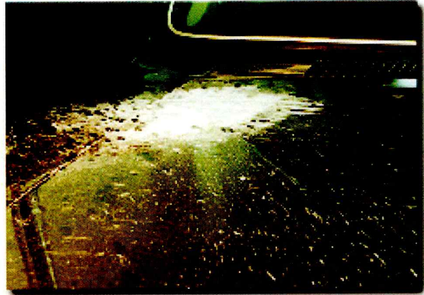
C-5 These spots are from industrial overspray, which usually can be removed through the detailing process.
