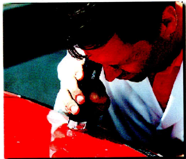
B-1 A low-power magnifier will reveal the depth of surface defects.
