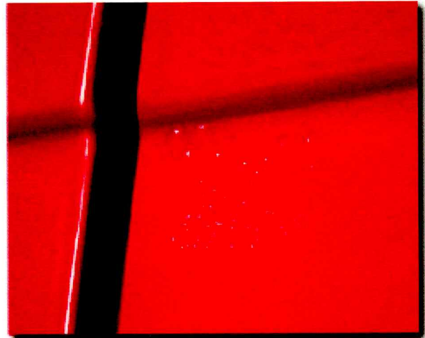
C-3 Silicone contamination that shows in the final topcoat cannot be removed by detailing.
