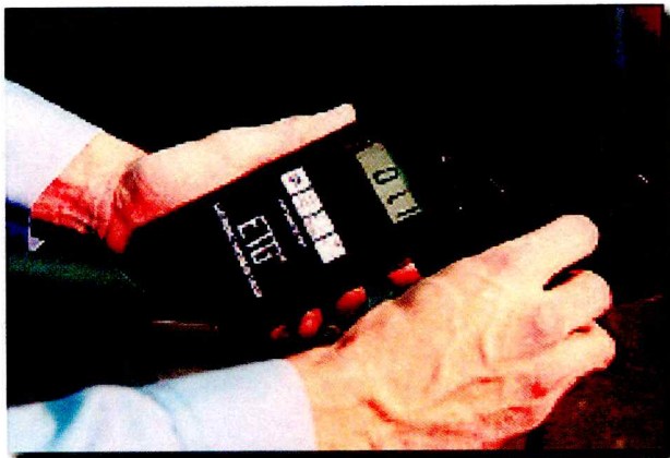
B-2 A digital film thickness gauge is necessary for the small readings that must be taken during detailing.
