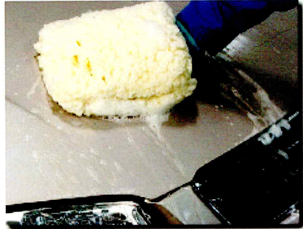
A-3 Car wash soap and water does the work, then the vehicle is rinsed off with plain water.
