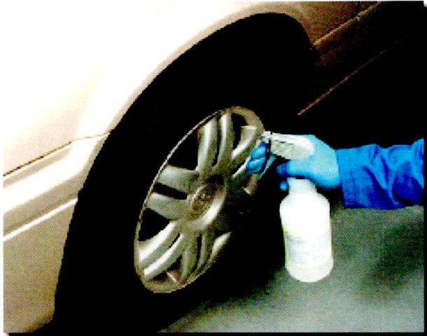
G-4 Use a dressing designed for tires, but if the application is in a collision repair facility, stay away from silicone-containing dressings.
