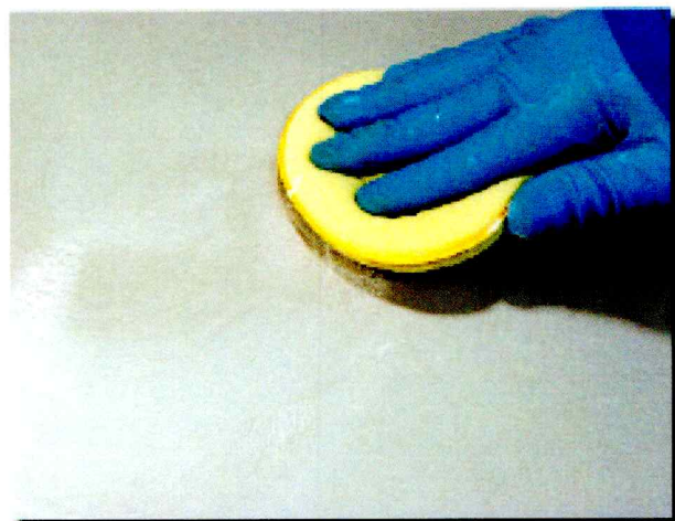
E-3 Wax is usually applied by hand, with a circular motion, and then wiped off after the surface glazes.
