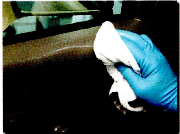
D-1 Conditioners provide moisture to porous materials to prevent fading, drying, and cracking.
