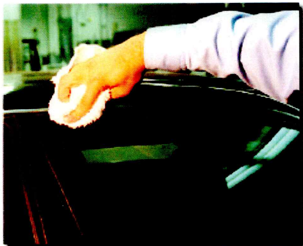
E-2 When cleaning glass, make sure to clean the top edge of the door glass, which is often missed.
