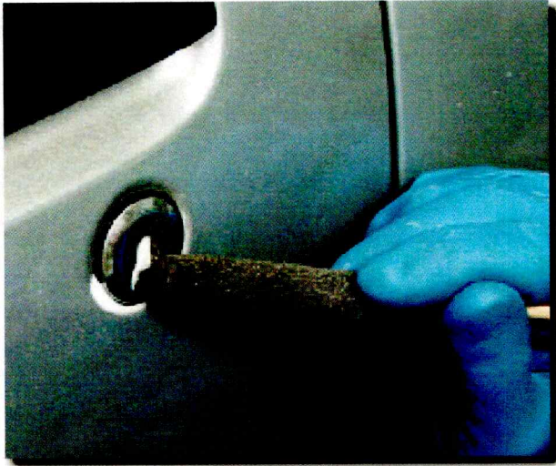
F-1 During final exterior detailing, look under and in small areas for remaining polish or other buffing materials.
