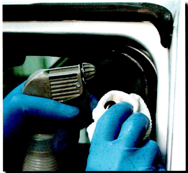
E-1 Condition weatherstripping with a dressing designed for exterior vinyl.
