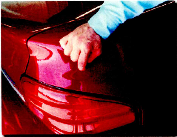
C-4 Light scratches can be removed, but if it can be felt with a fingernail it is too deep to be removed by detailing.
