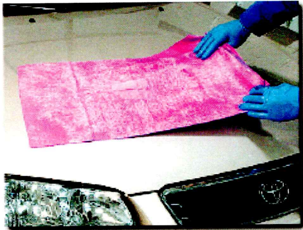
A-4 A preferred method of drying is to lay the towel or chamois down flat and drag it across the surface.
