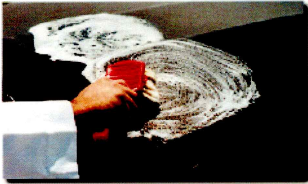
G-1 Vinyl tops are porous and may be textured, so use a circular cleaning motion to ensure all the dirt is removed.
