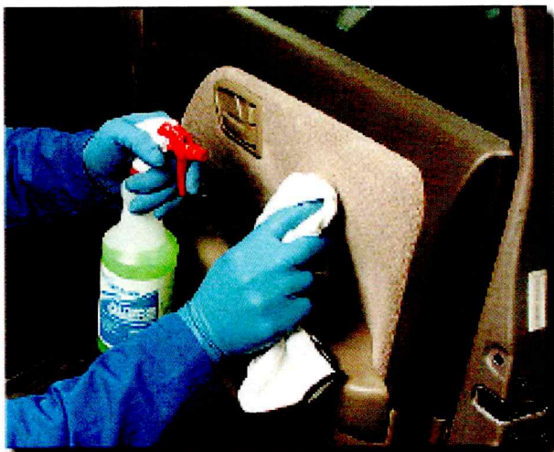
D-2 A common cleaning material for detailing is a solution of all-purpose cleaner.
