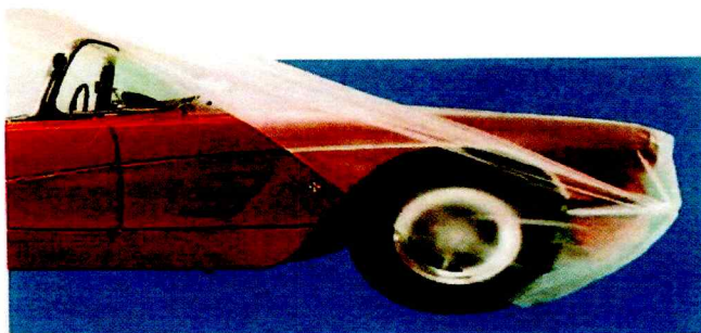
Figure 13 ♦ Overspray protective sheeting. (Courtesy of
