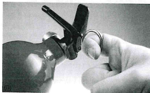
FIGURE 14-12B Release the pin on the fire extinguisher.
