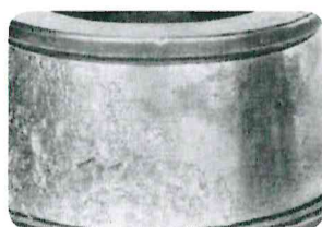
Inner race damage from misalignment. (fig. 5)
