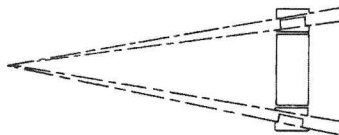
Lines extending the tapered roller bearing's inner and outer races will eventually coincide. (fig. 2)
