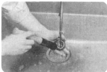
Rinse the bearing in clean solvent. (fig. 7)
