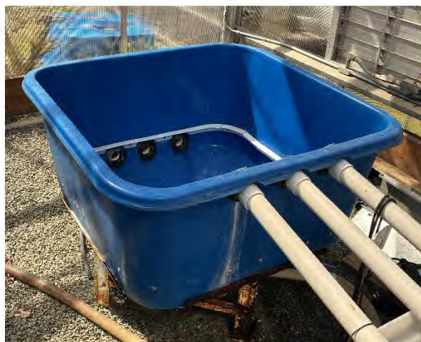
Tank #2 Dimensions: 3.5' x 3.5' x 2' Gallons: 180 Condition: Good
