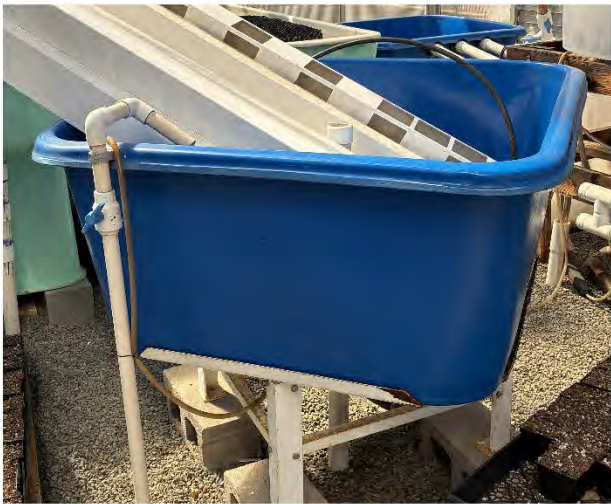
Tank #5 Dimensions: 3.5' x 3.5' x 2' Gallons: 180 Condition: Good
