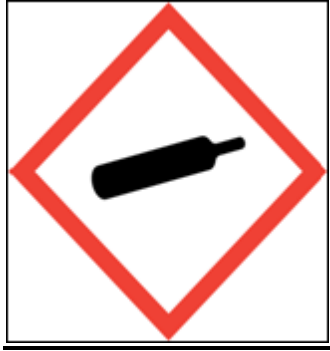
Gas under pressure
