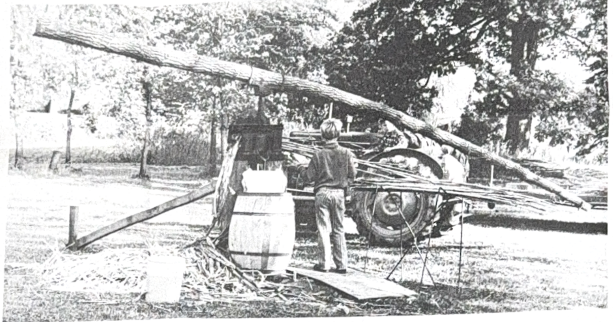
...the sorghum cane is pressed in this tractor-powered cast iron press....
