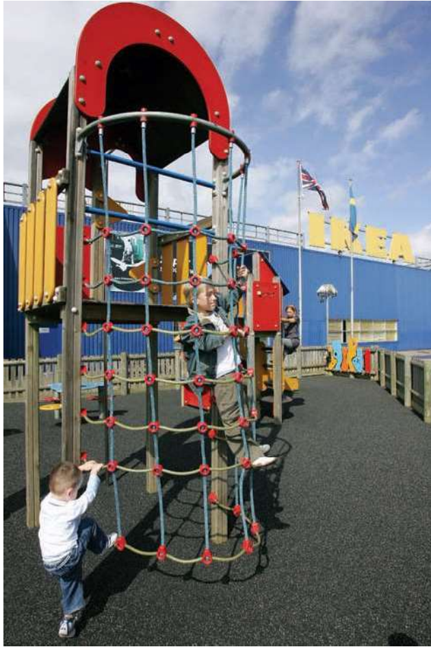
Nike Grind. Making this athletic playing surface from recycled sneakers and sneaker manufacturing waste saved resources and energy. (Courtesy of NIKE, Inc.)
