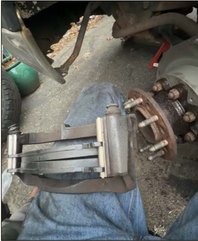
front rotor and brakes replacement
