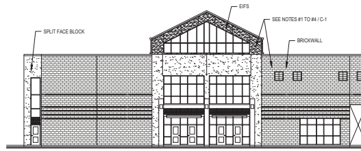
2 NORTH WEST INNER ELEVATION SCALE: \frac{1}{32}'' = 1'-0''
