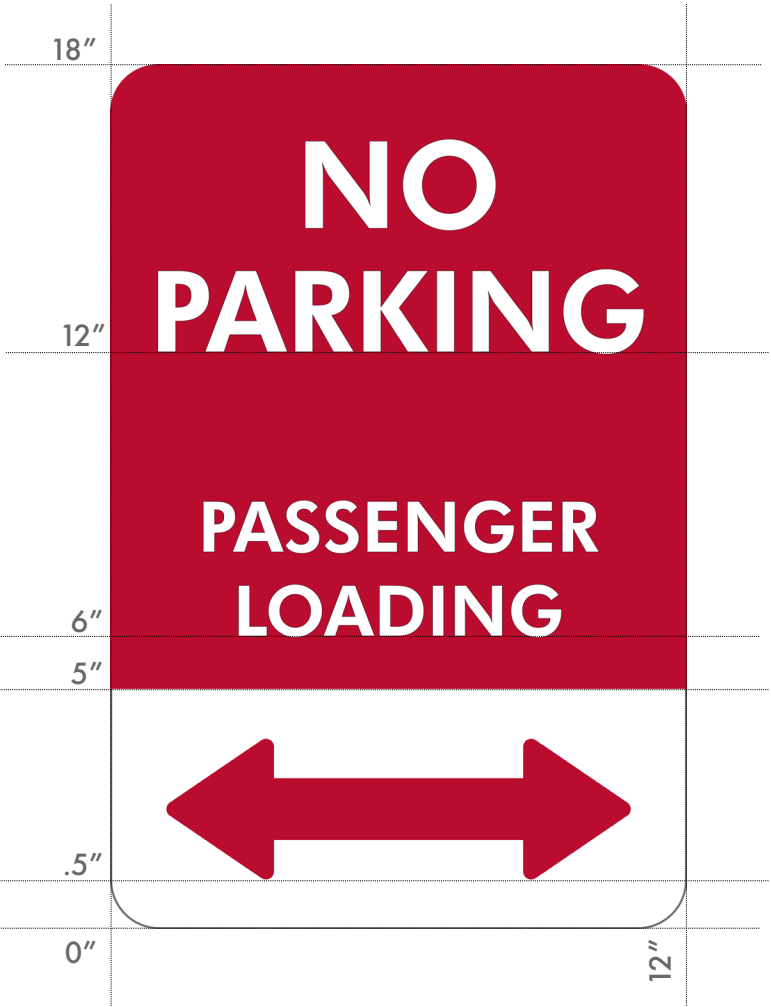
SIGN 1 PASSENGER LOADING - DOUBLE ARROW
