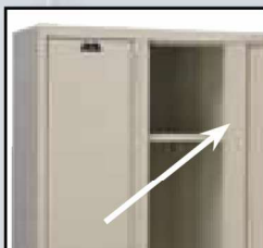
STANDARD A 3" wide 18 gauge full height door stiffener spot welded to the inner door face and MIG welded to the hinge side as well as to the top and bottom door flanges providing a rigid torque-free door. A 1-1/2" wide stiffener will be furnished for 9" wide Marquis doors.
