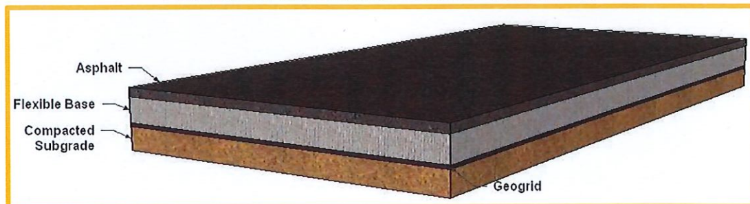
FIGURE 4.2: OPTION 2 FLEXIBLE PAVEMENT TYPICAL SECTION
