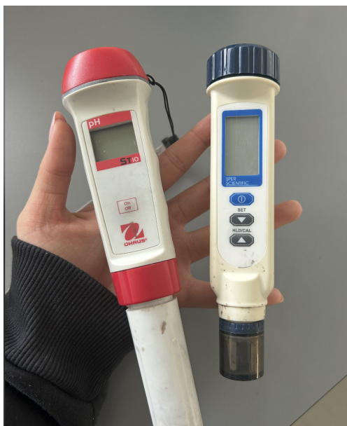
Figure 1: Illustrates the pH and conductivity pens used.
