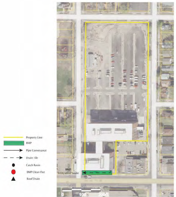
BMP Location and access points for inspection of underground infiltration facility
