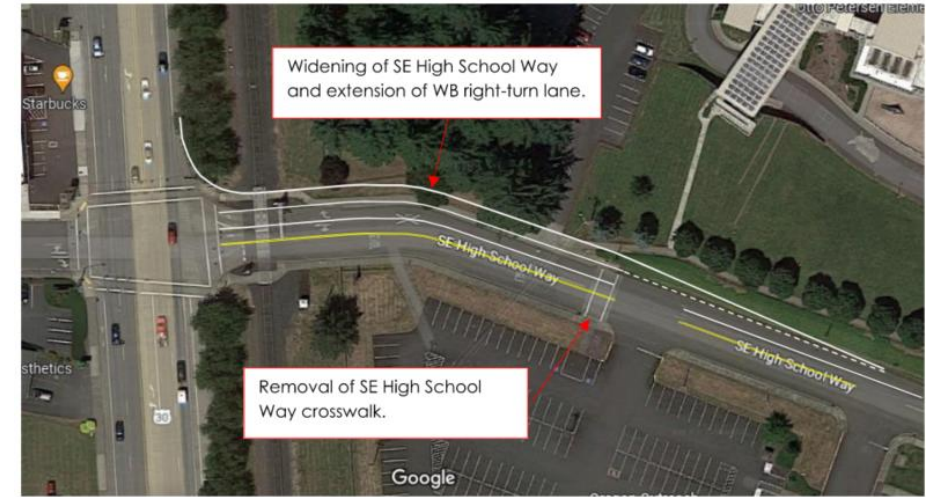
Exhibit 1 – US 30/SE High School Way Intersection Conceptual Mitigations (For illustrative purposes only)
