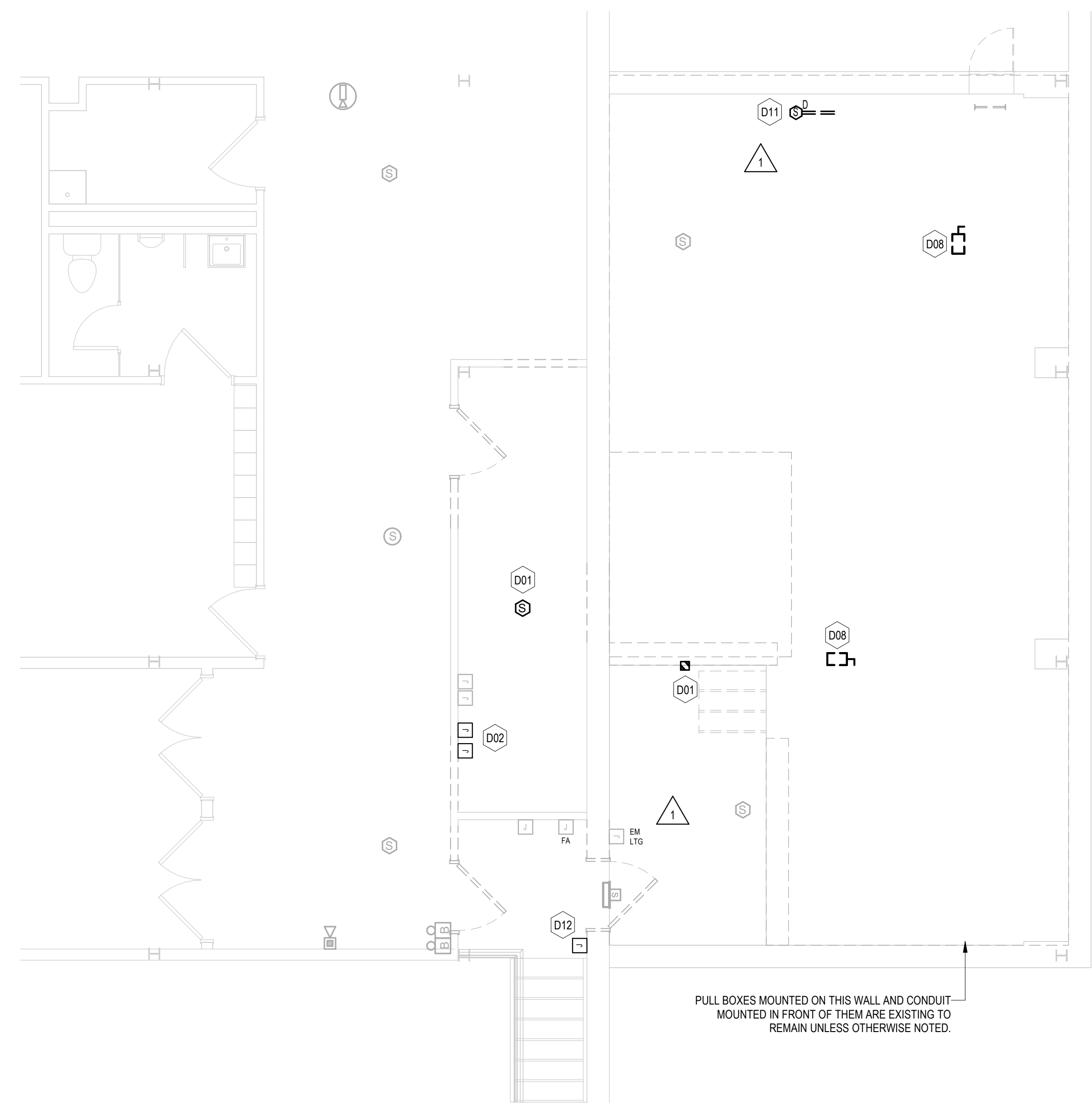
1 PARTIAL LOWER LEVEL DEMOLITION PLAN - POWER 1/4" = 1'-0"
