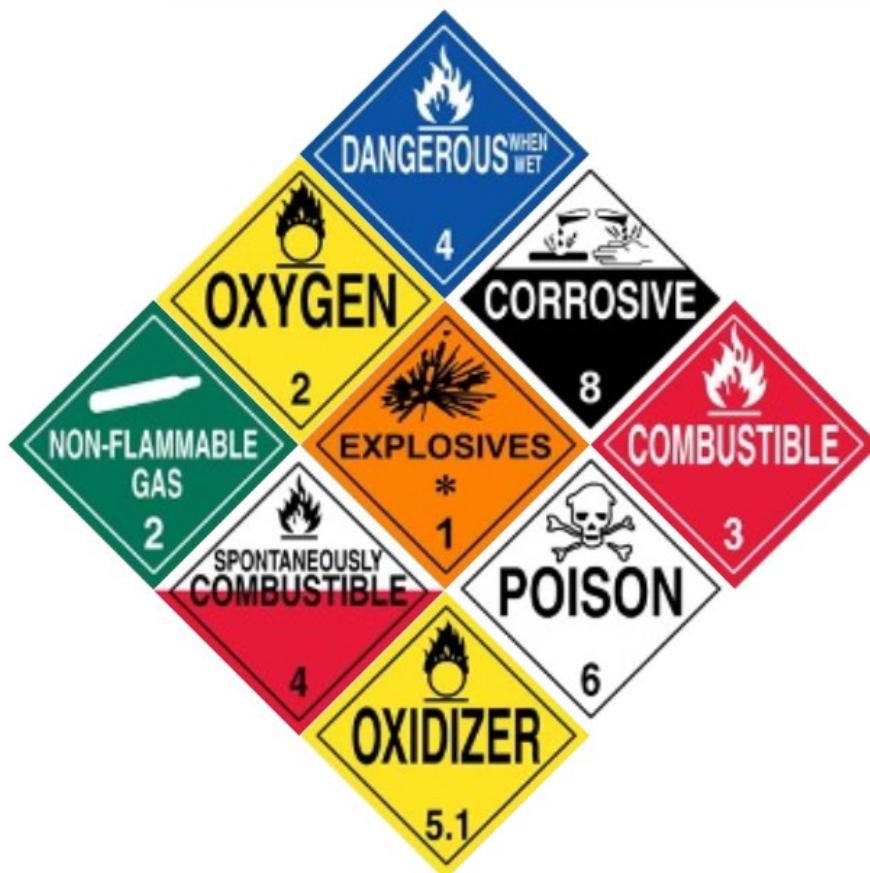
Figure 3: Examples of DOT labels for the various chemical hazards.
