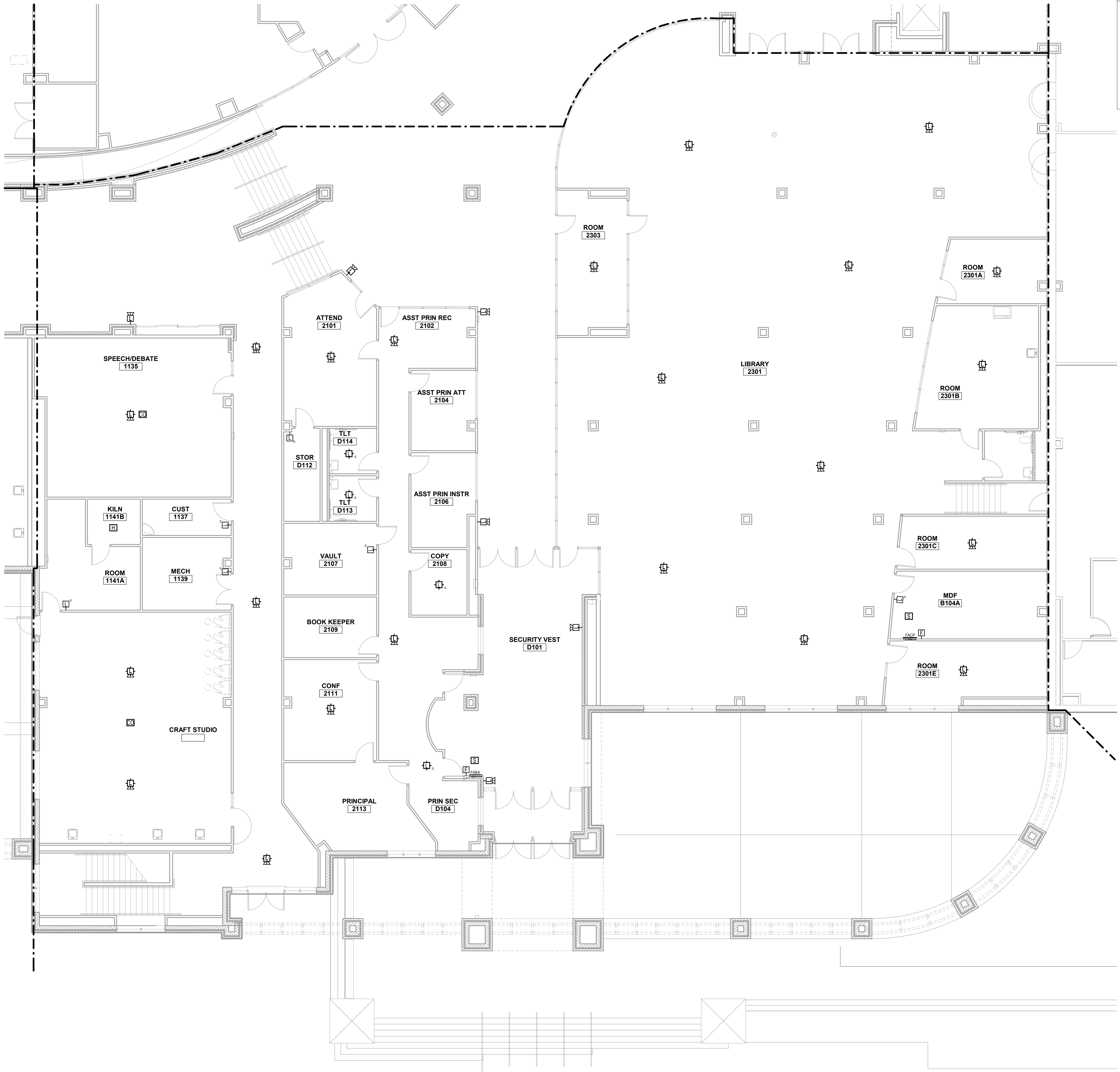
1 FIRE ALARM FLOOR PLAN - LEVEL 1 - AREA F 1/8" = 1'-0"
