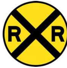
Figure 7-3. Railroad Crossing Advance Sign.
