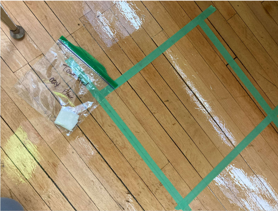
Figure 2: Example of a floor sample within one of the classrooms.
