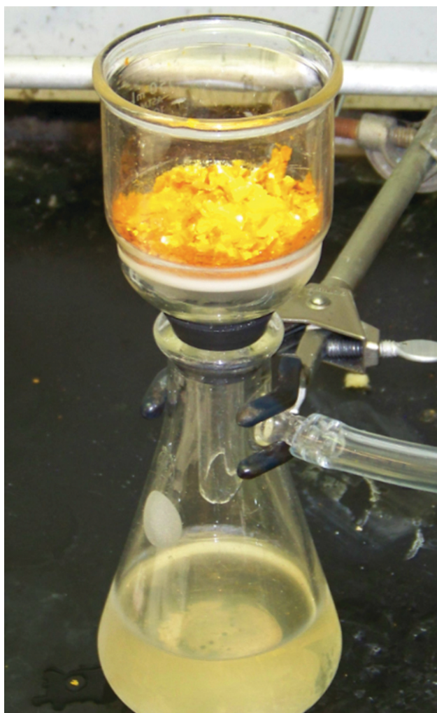
FIGURE 4.17 Precipitate may be removed from a reaction mixture by filtration.
