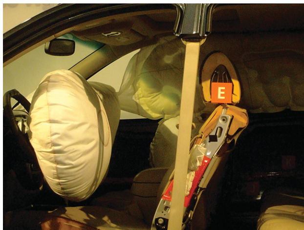
FIGURE 4.12 Airbags deploy upon impact to minimize serious injuries to passengers. (credit: Jon Seidman)
