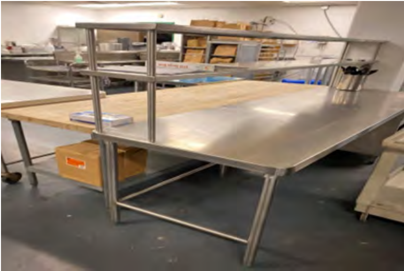
FS-4: Wood surfaces are not allowed in a kitchen unless it is being used in a specific task as part of baking or other dough processing. Wood surfaces are difficult to maintain in the long term and they require frequent oiling and other maintenance. If not oiled the wood shrinks and splits causing health code violation since the gaps fill with debris and it is not possible to clean and sanitize. Replace wood table tops with stainless steel built to NSF standards.
