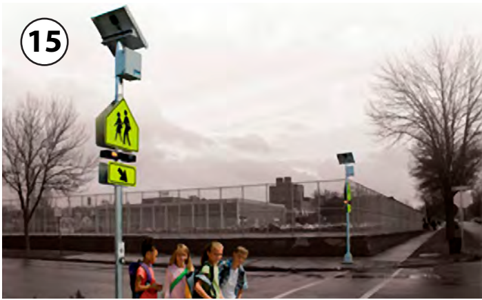
Rectangular Rapid Flash Beacons increase yield compliance at uncontrolled crossings.
