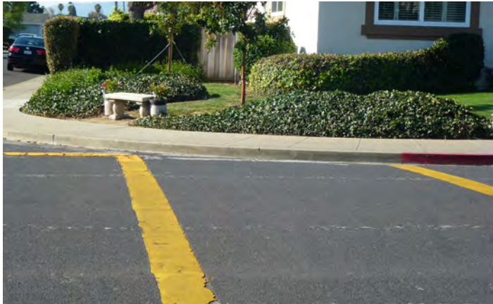
Wide turning radii at intersections can result in higher vehicle speeds.
