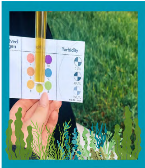
(Above) The turbidity of the water is the cloudiness of it. Turbidity matters in an ecosystem because if it is too cloudy, it prevents sunlight from reaching aquatic plants, therefore affecting photosynthesis and the overall survival of aquatic plants.
