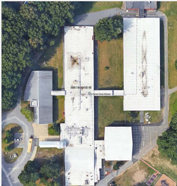
Roof Photo #17: AS is around roof top equipment and ponding water.
