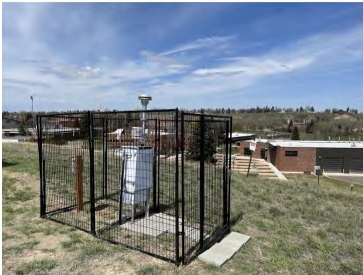
Figure 2: a particulate matter monitoring site installed this year on MSU Northern's campus in Havre; this site will look identical to the new equipment installed in Great Falls
