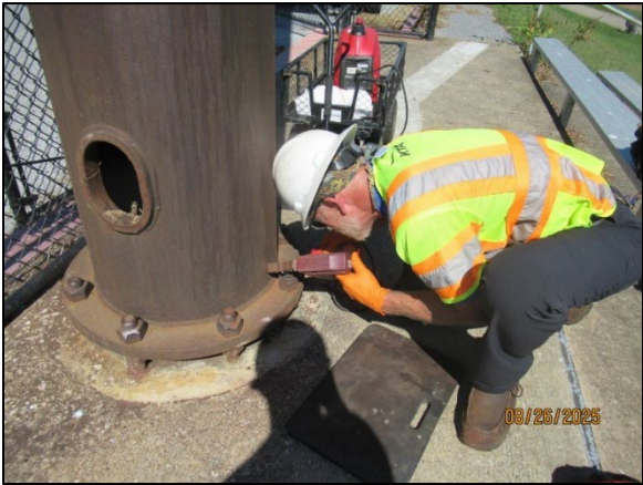
Non-Destructive Weld Examinations Magnetic Particle Testing (Left) and Ultrasonic Testing (Right)
