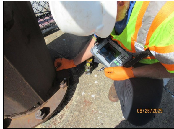
Non-Destructive Weld Examinations Magnetic Particle Testing (Left) and Ultrasonic Testing (Right)
