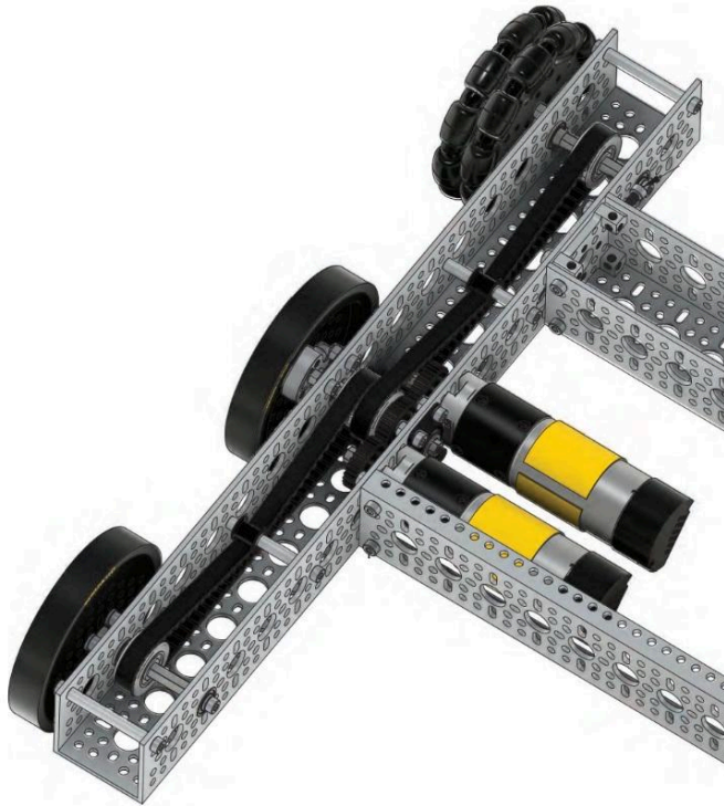
Example 1: Wheels being powered by belts off central gear
