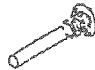
2 MALE CONNECTOR BOLT USED ON CABINET TO CABINET ATTACHMENT ALSO USED TO ATTACH SIDE PANEL TO CUT AWAY GLU LAM PANEL
