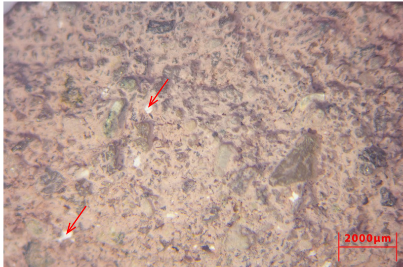
Photomicrograph of a polished section before digestion with examples of lime nodules indicated by red arrows (incident daylight-balanced light, 10x magnification).
