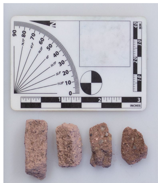
Photograph of a portion of the sample before acid digestion showing clean breaks on the left and weathered faces on the right (fluorescent light, color corrected).
