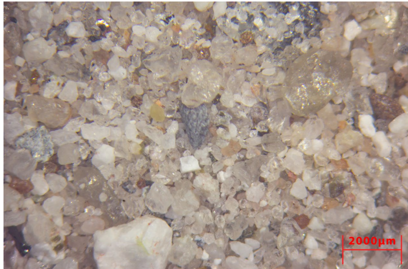
Photomicrograph of the extracted aggregate before sieving (incident daylight-balanced light, 10x magnification).
