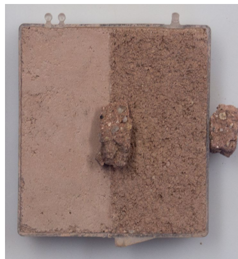
Portions of the tested sample compared to a tile of colored Ecologic™ Mortar (fluorescent light, color corrected).
