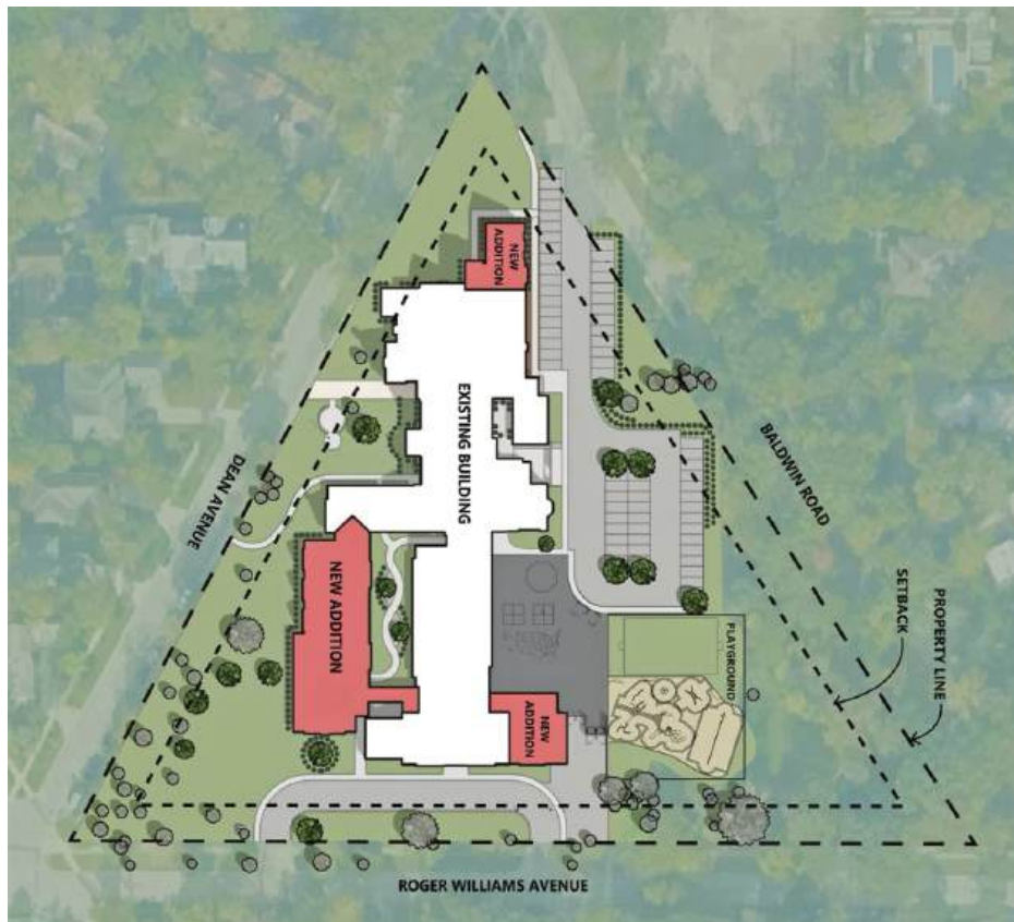
2024-25 Ravinia School additions: new kindergarten (left), lunch server room (right), and stairs & elevator (top).
