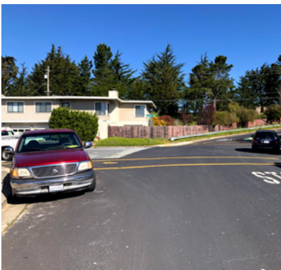
Figure 10. Vehicles parked at crosswalk ends obstruct the view of crossing pedestrians at Alhambra Rd and Ponderosa Rd.
