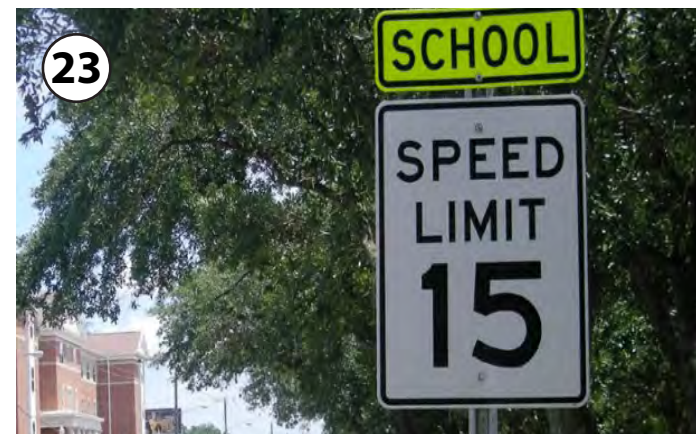
23 15 or 20 MPH school speed limit ordinances can further reduce traffic speeds in school areas.
