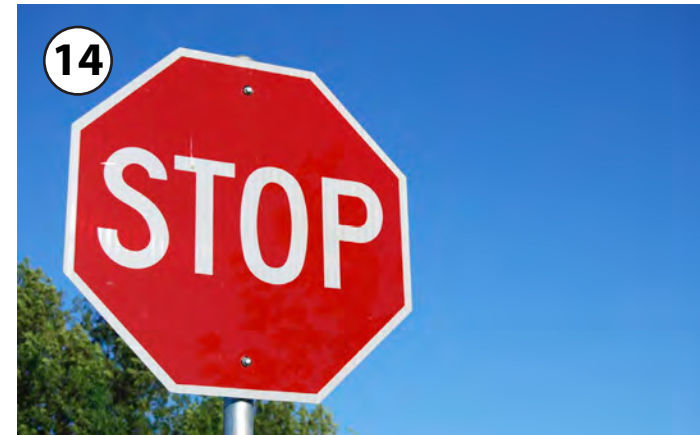
14 STOP signs may be installed where pedestrian volumes or other safety considerations warrant.
