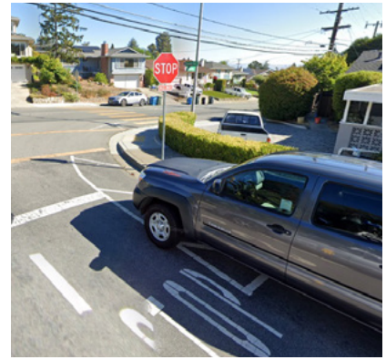
Figure 6. Vehicle parked over painted curb extension at Emerald Hill Rd/Jefferson Ave
