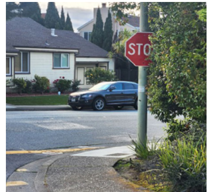
Figure 3. Obstructed stop sign at Green Hills Dr/Laurel Ave.
