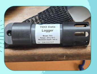
This is a temperature logger, it measures water temperature as it goes down and sends it back to the boat.
