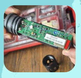
The logger can record data continuously as it descends through the water, measuring the temperature of the entire water column.
