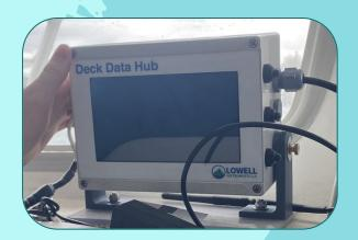
This is the data hub. It wirelessly connects to the sensors, receives real-time data, and clearly displays it on the screen for easy viewing.
