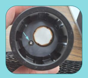
This is a newer version of the temperature logger; it uses this metal pin to measure the temperature of the water.
