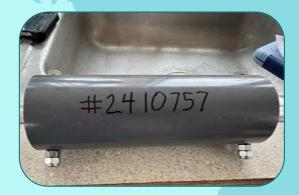
The logger is placed in a protective PVC case to prevent it from being damaged.
