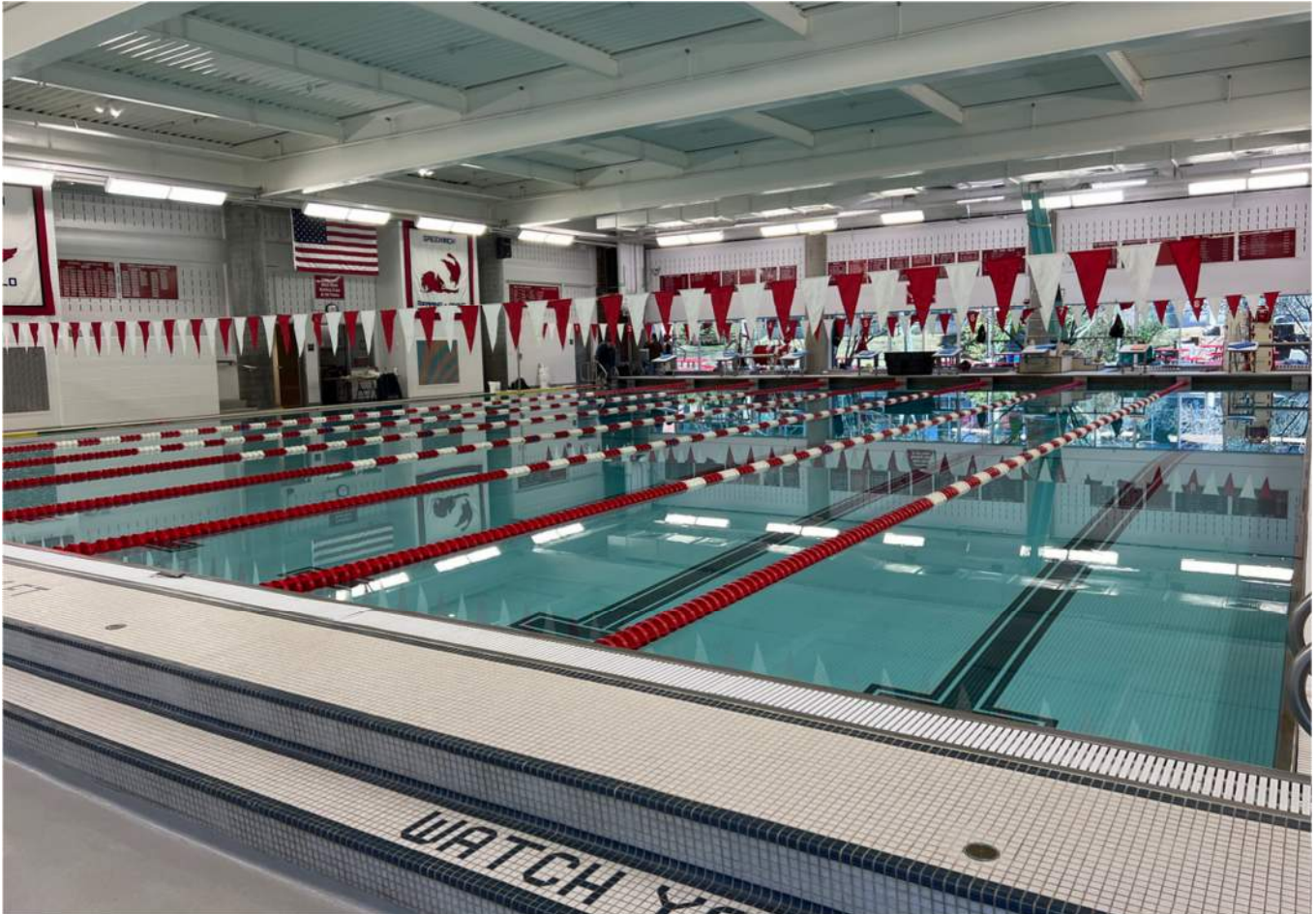
Photo 1 (Above): Overall view of pool from shallow-end. Pool edge is built up with a bulkhead curb and steps to form a recessed gutter on the touch walls.
