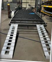
Students in Patchogue-Medford's Construction Trades program are building reusable float bases for special trailers. These trailers and bases are designed for our homecoming parades, with frames that make it easy to put up and take down different float designs each year. This creates a lasting solution for future parades while giving the students hands-on practice with the construction skills they're learning.
