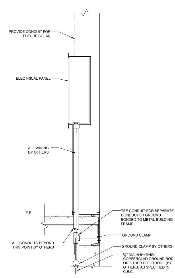
1. SIZE OF CONDUCTORS SHALL COMPLY w/CEC.A 2. BOND SEPARATE CONDUCTORS FROM GROUND ROD TO ELECTRICAL PANEL & METAL BUILDING FRAME (CEC). IN ADDITION TO THE DETAIL SHOWN ABOVE, BOND THE ELECTRICAL GROUND TO METAL WATER PIPE EMBEDDED AT LEAST 10' INTO THE SOIL IF AVAILABLE (CEC).
