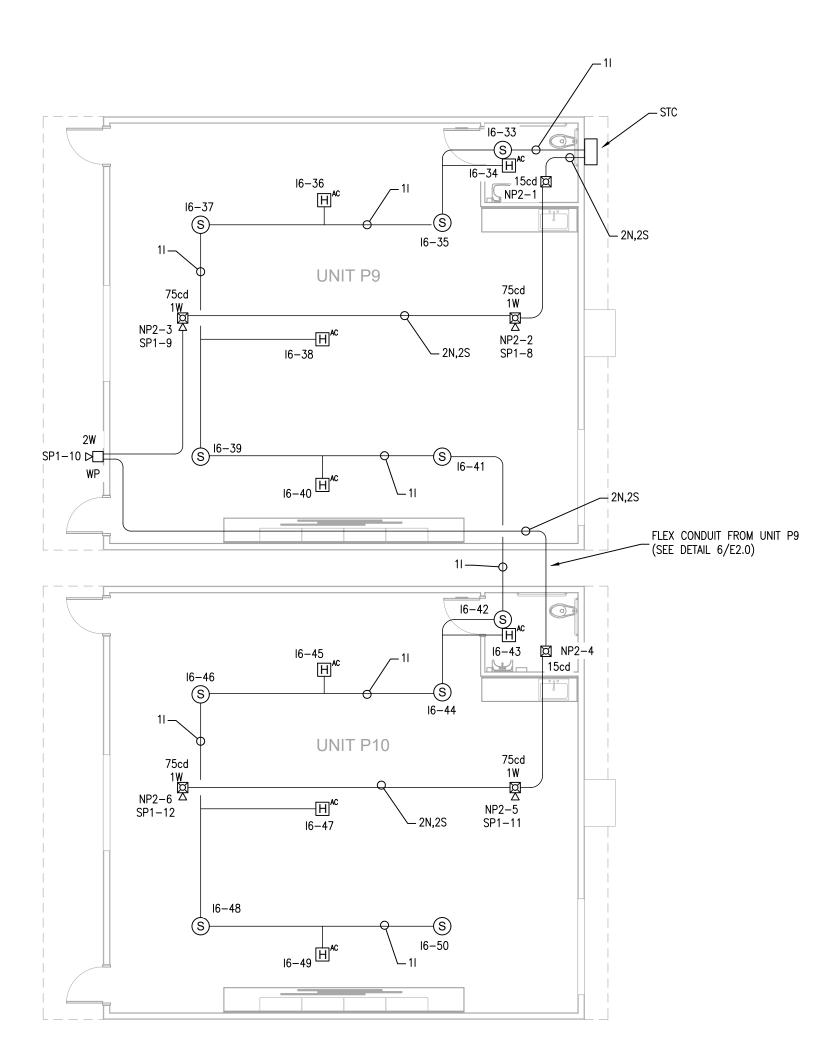
**FIRE ALARM PLAN - RELOCATABLE CLASSROOM** SCALE: 1/8"=1'-0"
