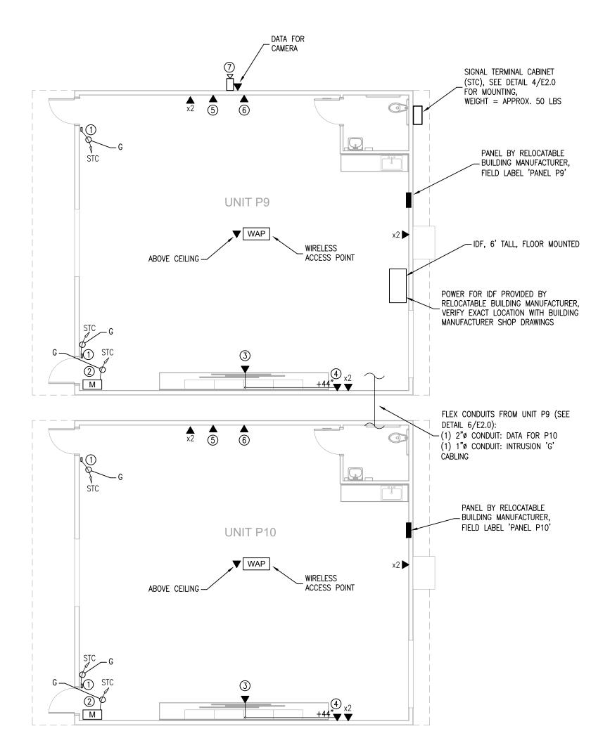
**SIGNAL, DATA, & INTRUSION PLAN - RELOCATABLE CLASSROOM** SCALE: 1/8"=1'-0"
