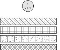
REFERENCE KEY TO SITE DETAILS DETAIL I.D. NUMBER (TOP) DETAIL SHEET NUMBER (BOTTOM) PROPOSED MEDIUM DUTY RECLAIM AND REPAVE PROPOSED CONCRETE VALLEY GUTTER 9 C2.01 PROPOSED CONCRETE SLAB REPLACEMENT
