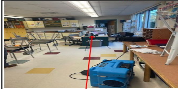
Photo 1: View of typical classroom spore trap air sampling. HEPA filtered fan unit present operated off-hours.
