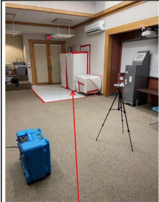
Photo 1: View of room 203 closet containment with decontamination chamber during Assembly room 203 background spore trap sampling.
