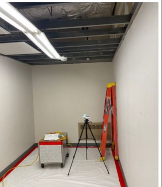
Photo 4: View of room 203 storage closet containment during post remediation spore trap sampling. Surfaces and heater fan cleaned free of suspect mold and debris.
