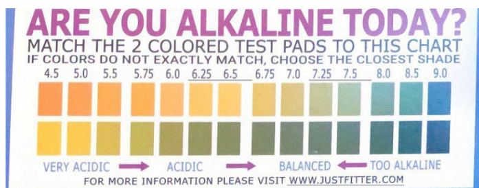
Figure 7: Raw picture of pH key used to determine RGB values of each pH value.
