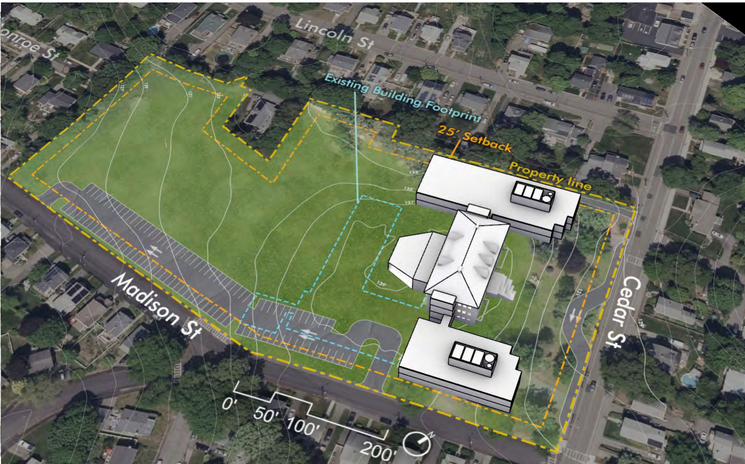
'Addition/Partial Renovation' – Site plan
