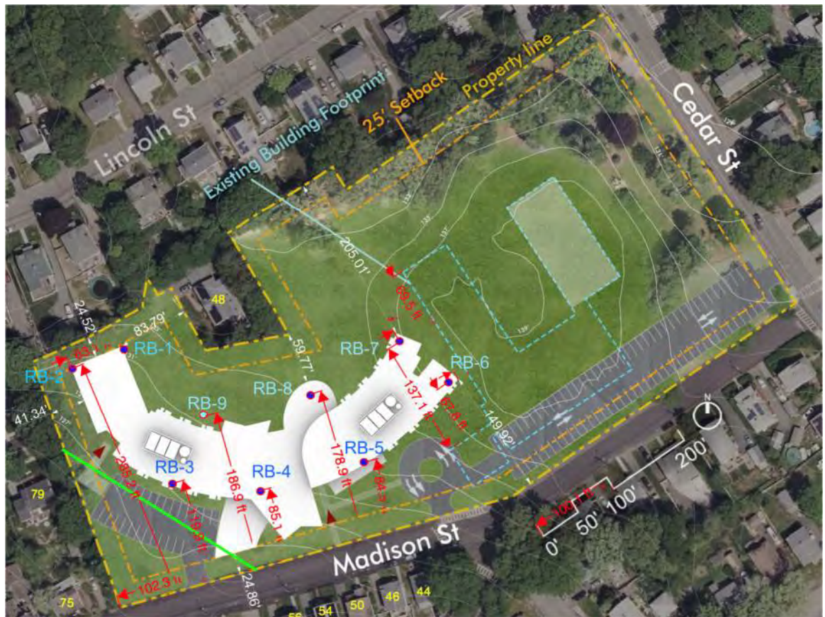
FIGURE 10 – Approximate Boring Locations at Oakdale Elementary School, Dedham, MA (Field Program: 18 & 21 August 2023) (Note: the locations were field measured by field engineers from Reliance Engineers).
