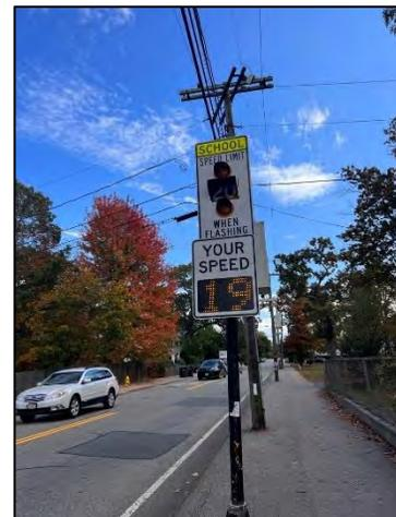
**Photo 1. Flashing Speed Limit and Radar Speed Signs along Cedar Street**
