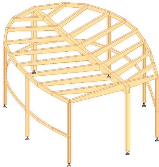
Figure 1 – Media Room Timber Framing Isometric
