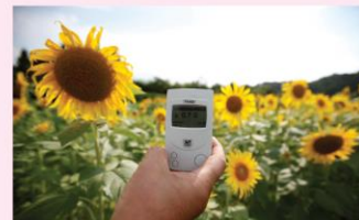
▲ Figure 2 A Geiger counter, measuring radiation levels in a crop of sunflowers. The sunflowers are being used for bioremediation of soil contaminated with radiation
